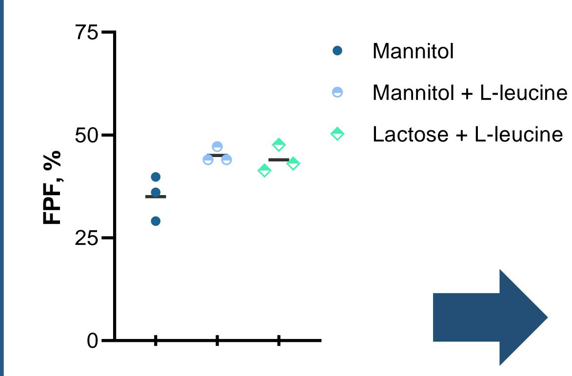
Residue in the capsules and fine particle fraction (FPF) of the spray dried formulations with mannitol or lactose matrix after the addition of L-leucine (+) in comparison to the spray dried mannitol-based formulation without L-leucine (-).
