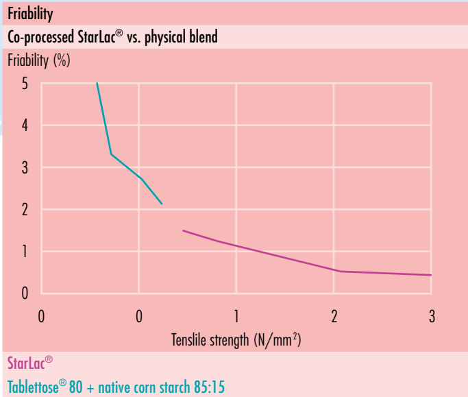
Figure 11: Friability of tablets produced either with StarLac® or its corresponding physical blend.
