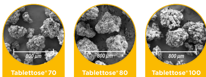
Figure 6: SEM images of MEGGLE's Tablettose® by ZEISS Ultra55 FESEM (U=5 kV; Au/Pd sputtered).
