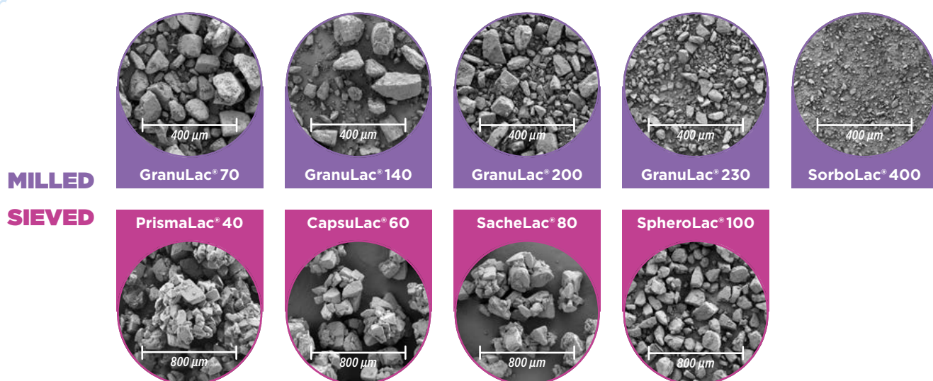
Figure 6: SEM images of various milled and sieved MEGGLE lactose grades by ZEISS Ultra 55 FESEM (U=5 kV; Au/Pd sputtered).
